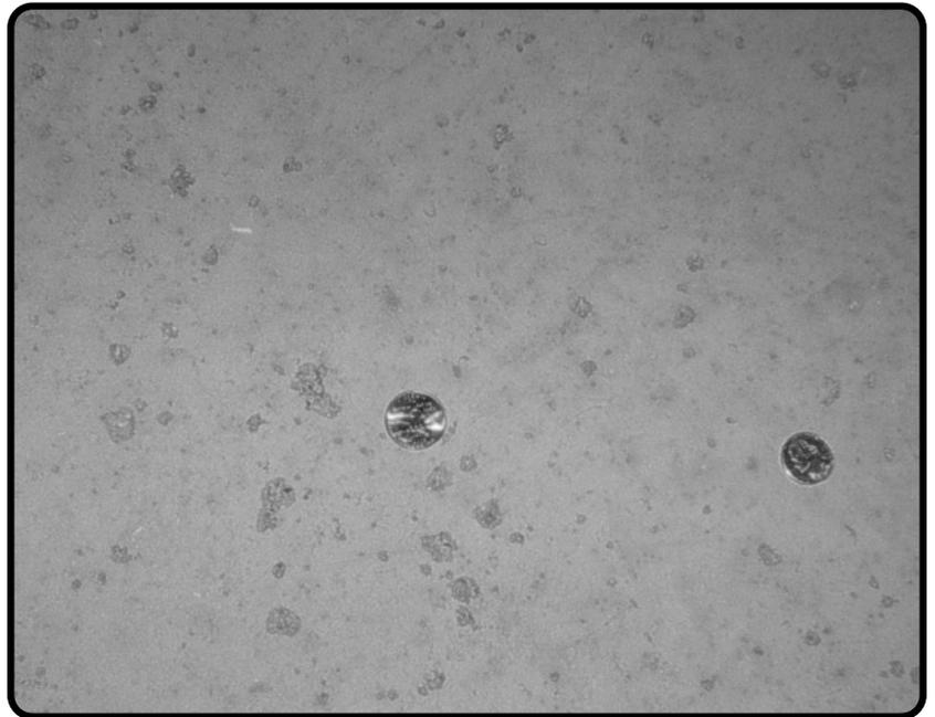
Use the proper concrete mix. Use a concrete mix with workability suited to the type of mechanical placing and finishing equipment to be used. The greater the slump, the more likely small, lighter weight particles will be displaced to the top of the surface.
